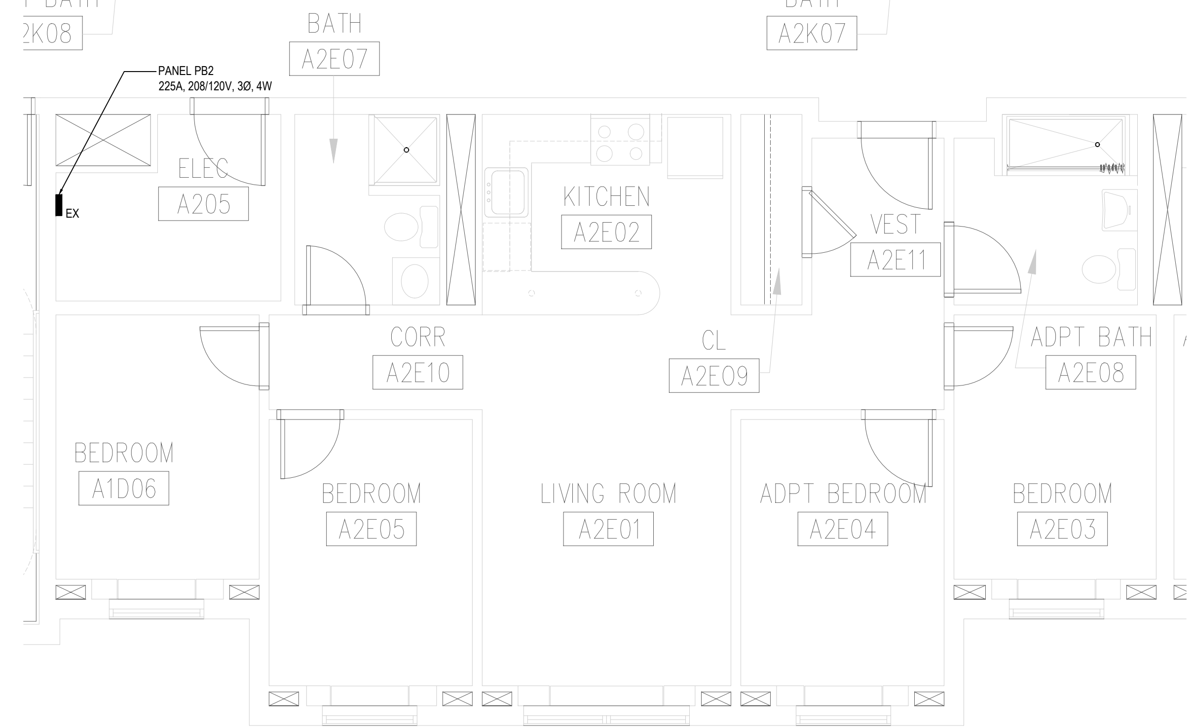
2 SECOND FLOOR PARTIAL PLAN - DEMOLITION 1/4"=1'-0"
